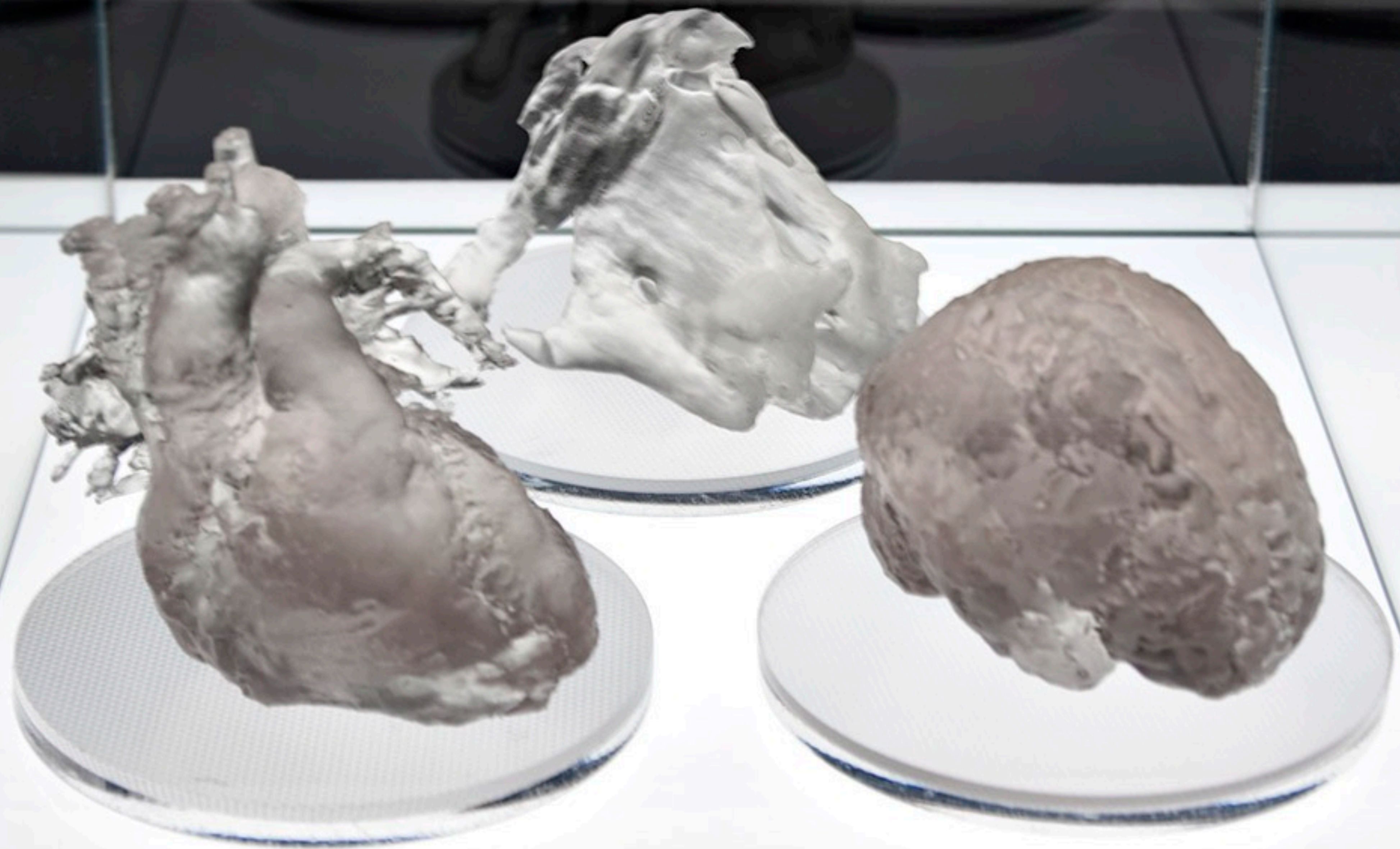
Specific mergers were created for organ segmentation to print in flexible resin. Left: Heart – 1 male x 1 female. Center: Voice Box – three subjects, no further data. Right: Brain – 1 female 65 years old x 1 male 19 years old.
