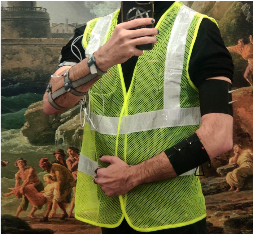
Figure 26: Vest fit test. [right arm(L)]: EMG sensor straps. [left arm(R)]: electroshock sleeves. [vest center-L]: microcontrollers. [vest center-R]: TENS device
